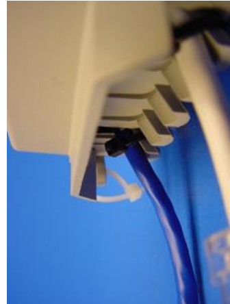
Cable entry with protective shroud and cable tie lugs
