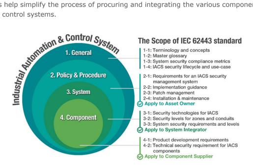
Figure: The ISA/IEC 62443 standards define procedures for implementing electronically secure IACS. This guidance applies to various stakeholders in the ecosystem.
