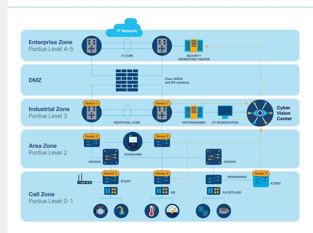
The placement of the sensors must make it possible to monitor the different interconnection points of the industrial system:
