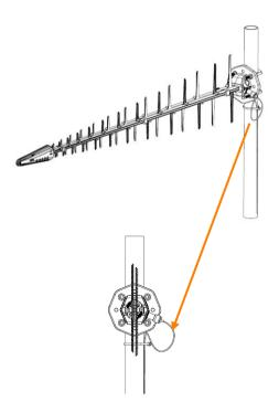
**Note**: The water drip loop is necessary for preventing water from running down from the antenna along the cable into the house and possibly the connected devices.
