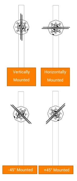
**Note:** Ensure that the connector is facing downwards when mounted in any orientation to minimise the risk of water ingress.
