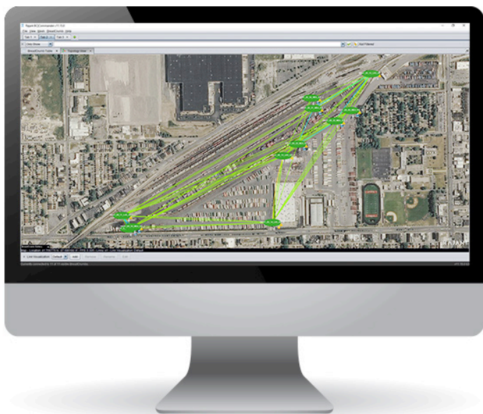
Rajant’s BCICommander mapping tool uses real-time GPS coordinates from the wireless radios to show the current links.
